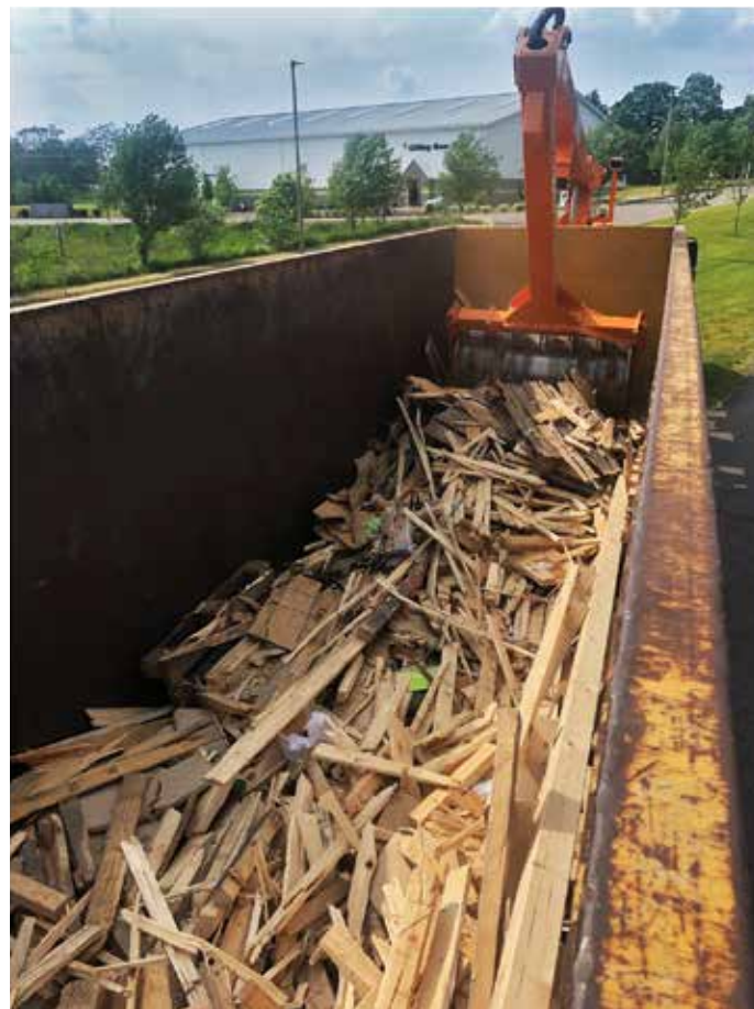
The Monster Smash truck compresses construction waste in a dumpster, reducing volume by one-third.
