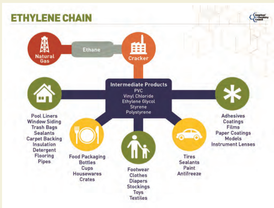
Figure 1. The process of cracking ethane into ethylene is critical to the manufacturing chain of dozens of products for which it is a feedstock. Source American Chemistry Council.
