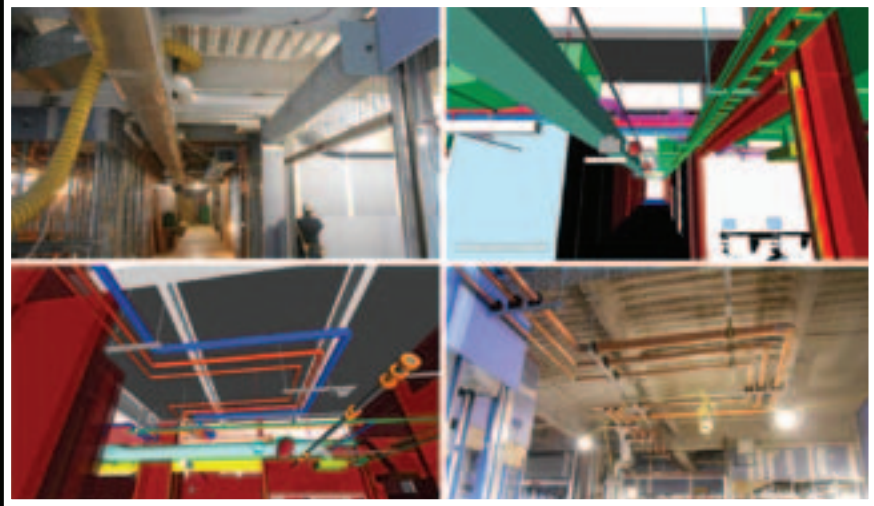
BIM models allow for coordination of multiple trades before field clashes occur. Image courtesy Astorino/Cannon.
