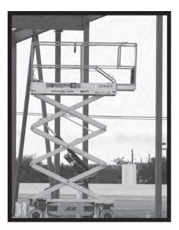
• Limit travel speeds according to workplace conditions, such as holes in the deck or un-level surfaces.
