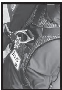
off point at least 15.5 feet above the next lower level. Shock absorbers built into the system can reduce this level to level distance. Keep in mind that certain tie-offs can reduce the static line or lanyard strength.
