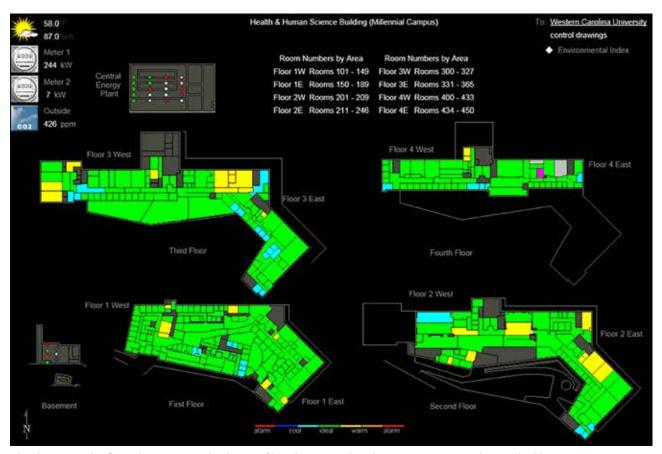
This thermographic floor plan was a good indicator of how heating and cooling was operating in the HHS building.
