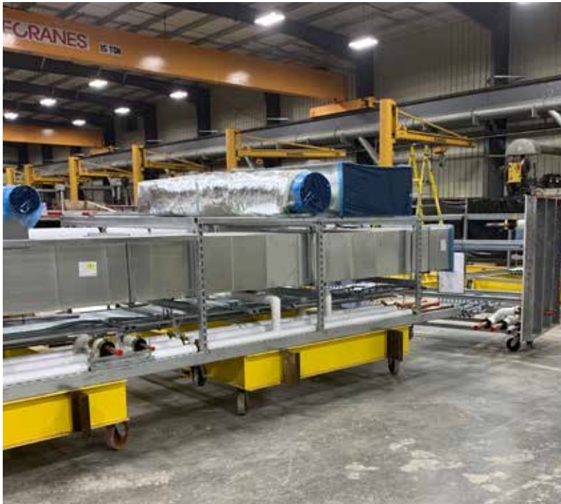
Racks were prefabricated individually in the shop to include all of the mechanical and electrical distribution, then fireproofed and sheathed in drywall. Photo by W. G. Tomko Inc.
