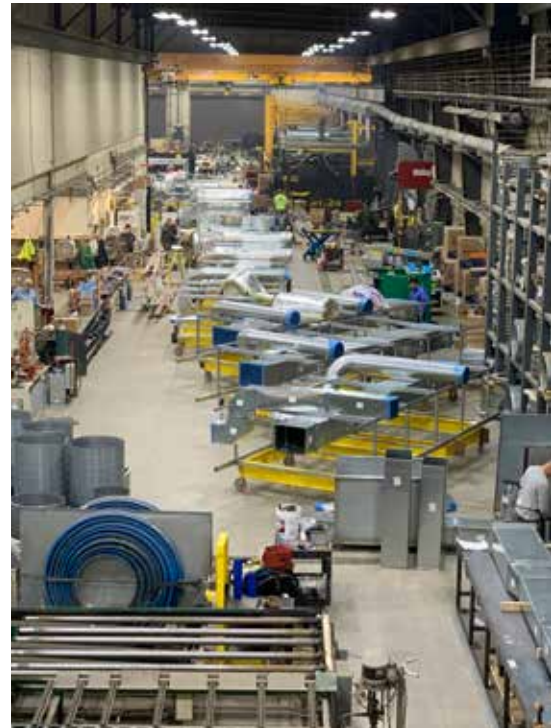
Fabrication of the corridor racks processed through 13 work stations in Tomko's shop. Photo by W. G. Tomko Inc.
