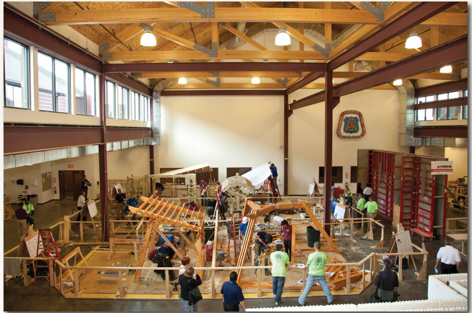
Clerestory windows allow ample daylight while freeing the perimeter walls for storage and training areas.
