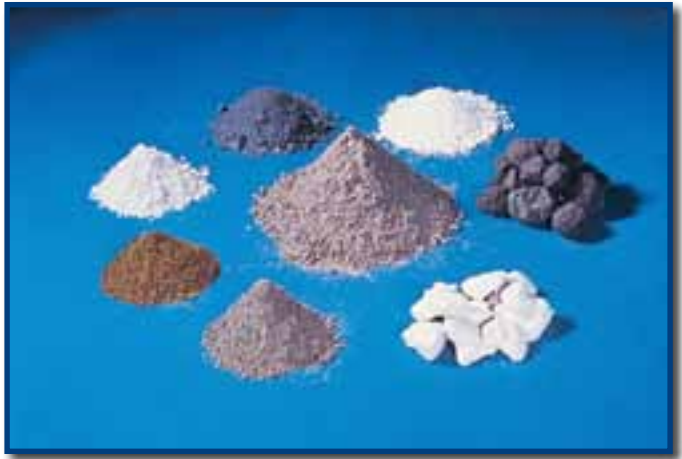
Shown is blended cement (center) surrounded by (right and clockwise) clinker, gypsum, Portland cement, fly ash, slag, silica fume, and calcined clay.
